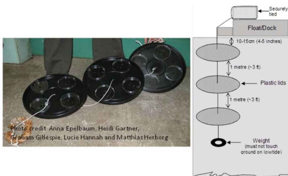
Figure 57. Collector plates used for monitoring invasive tunicates species in MABR.
