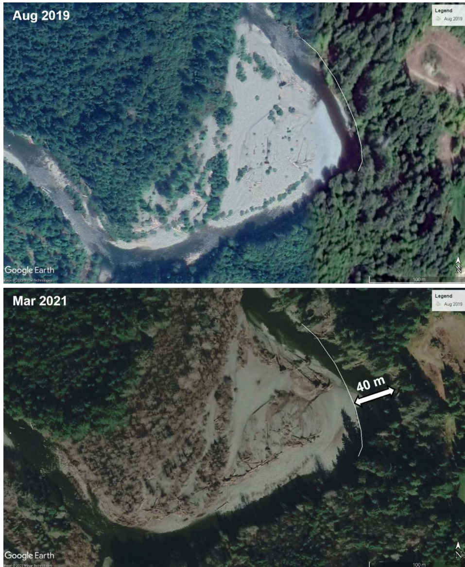
Figure 3.4 Rapid bank erosion at the downstream claybank (RK 6.3) from 2019 to 2021.
