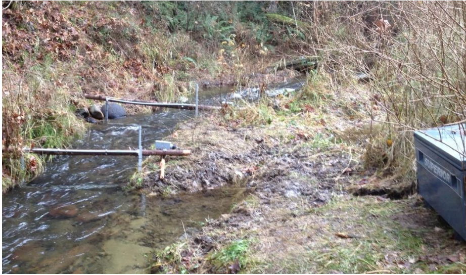
Figure 3. PIT tag detection array at Site 2 consisting of two pass-through antennas as well as a steel job box to house the reader and batteries (right).
